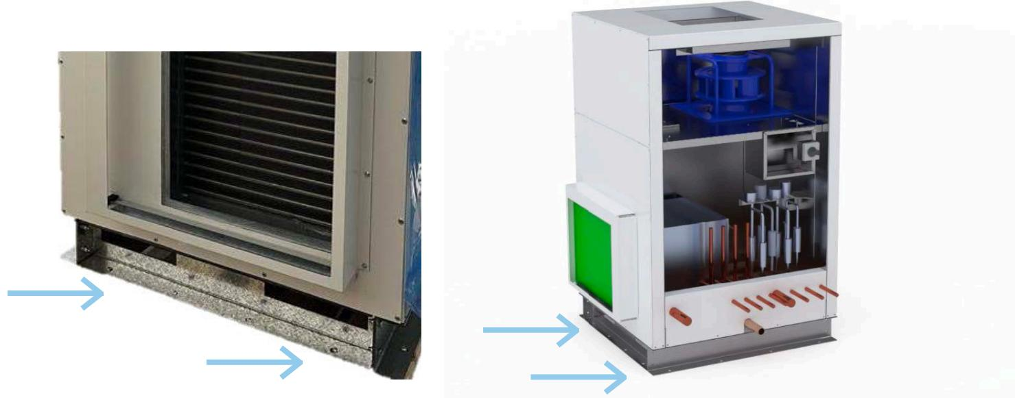
Accessory modules are shipped as a separate piece from the base unit. In some cases, a mixing box may ship coupled to the electric preheater or base unit and shall be lifted together only if a forklift can support the full length of both modules together.
