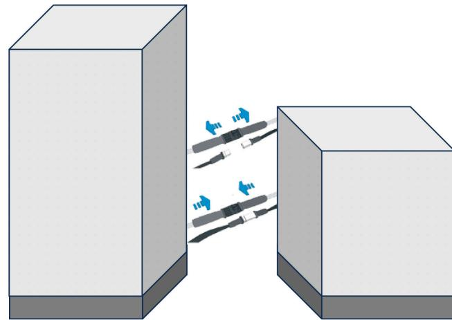
For unit-accessory configurations with either a post-heater and/or a mixing box + pre-heater combination, rear external connecting brackets are required to lock the split connections in place after initial joining has been completed. These external connectors shall not be used to close a gap between modules.
