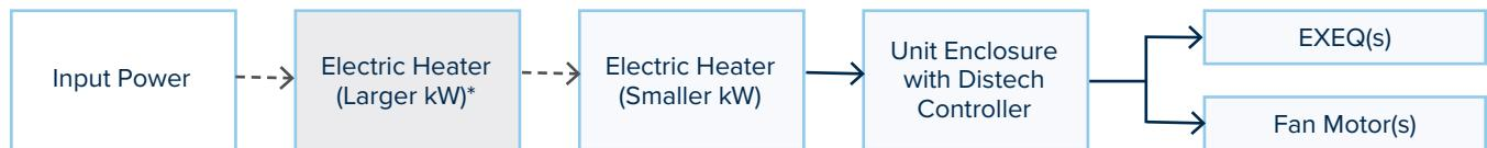
\* Using a second heater in a single-circuit power configuration is selected as a special only. Electrical ratings are not readily available. Single-heater in a single-circuit power selection is a standard offering.
