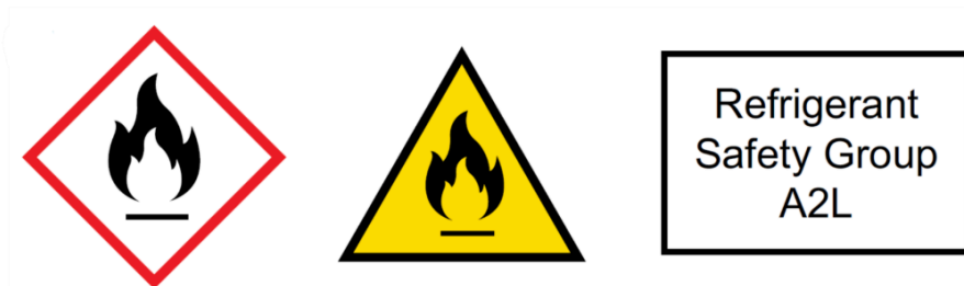
Figure 1. Flammable A2L refrigerant safety labels.
