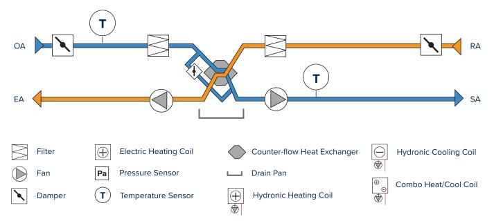
Ventum's unit controller takes advantage of the economizer option to provide "free" cooling (or heating) by bypassing outdoor air around the core and directly supplying air into the building when conditions allow.
