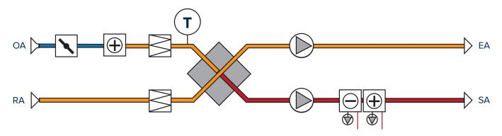
A SCR electric pre-heat coil ensures that the temperature entering the heat exchanger is maintained at a required minimum temperature. The pre-heat temperature sensor will come installed in the unit, positioned in the outdoor air stream. Pre-heat is controlled by a 0-10V signal.
