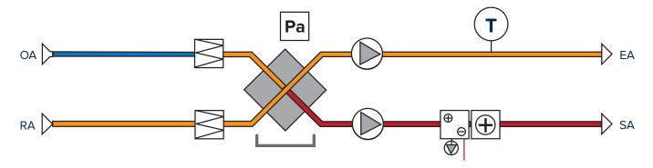
When frost accumulation is detected (based on the exhaust air temperature or by monitoring the pressure drop Across the Heat Exchanger), the supply fan ceases operation for 5\* minutes (\*adjustable), while the exhaust fan continues to operate and thaw the ice accumulation on the heat exchanger. After 5 minutes, the supply fan will resume normal operation until frost is accumulated again. This cycle repeats itself until minimum normal operating cycle time, 30\* minutes (\*adjustable).
