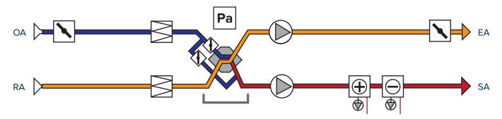
The heat exchanger can be protected against frosting by continuously monitoring the pressure drop across the heat exchanger. The actual pressure drop across the heat exchanger will be measured during commissioning, when there is no frost accumulated.
