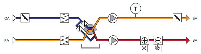
At temperatures below set value for the exhaust air temperature, the bypass damper will open to 100%. Thereby, the outdoor air passes around the heat exchanger and the return air passes through the heat exchanger. Due to the relatively high room temperature, this function will lead to the thawing of the frost accumulated on the heat exchanger. The post-heating coil should be sized accordingly to maintain the supply air temperature setpoint during defrost.
