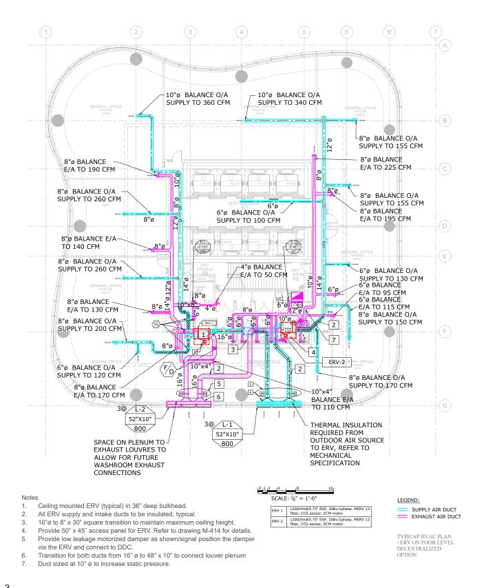
Schematics for Decentralized (M-1) and Centralized (M-2) HVAC Plan
